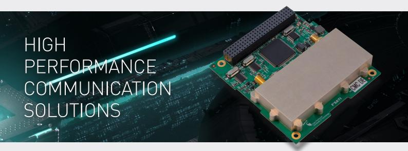
The PULSAR-TMTC is a compact telemetry and command radio designed for nanosatellite missions, compatible with the CubeSat standard with a CubeSat kit PC/104 form factor.
